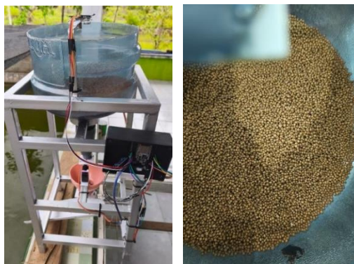
Figure 3. Hardware implementation of the automatic fish feeding system and feed storage hopper
