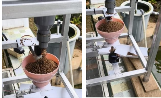
Figure 4. Load cell-based weighing container and feed dispensing mechanism into the pond
