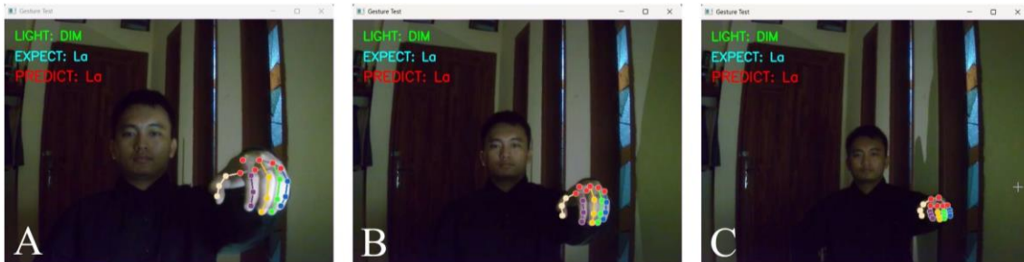
Figure 8. (A) "La" testing at 0.5-meter range and dim lighting, (B) "La" testing at 1-meter range and dim lighting, (C) "La" testing at 1.5-meter range and dim lighting
