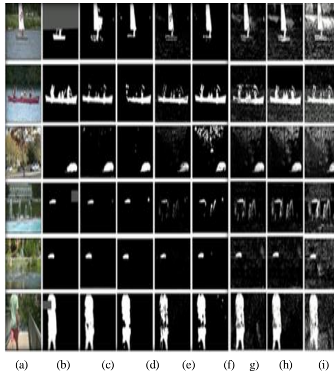
Figure 4. The visual comparison (a) original scene (b) ground-truth (c) The proposed FCM-CS foreground mask (d) SuBSENSE foreground mask (e) ViBe foreground mask (f) LOBSTER foreground mask (g) GMM foreground mask (h) KNN foreground mask (i) Codebook foreground mask
